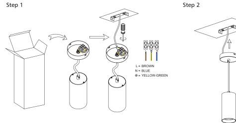
Proper alignment of mounting holes between back plate and mounting bracket, then lock them together with screw Take out the lamp, connect the corresponding polarities between the wires on the ceiling and terminal block by screwdriver.
